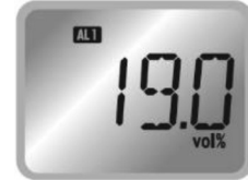
(Ex. AL1 alarm set value is currently set to 19.0vol%)
