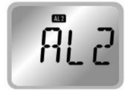
(2nd stage gas alarm)
