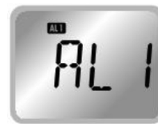
(1st stage gas alarm)
