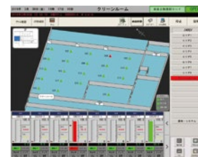
COD-203 Fixed-point monitoring based on installation drawings
